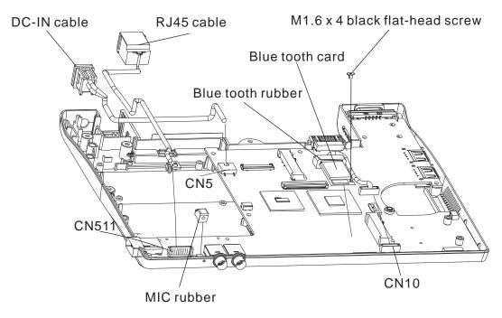
Figure 4-15 Removing the system board
